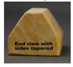
Between the square to be rounded into a ball and the sides tapered to narrow the face, cut in two notch cuts in the corner a little over an inch apart. These three steps are illustrated in the second block from the left in the first photograph.
