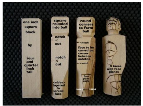
Three Version Face Study Stick begins as a one inch square by five inch basswood block. At the top of the block establish a square by making notch cuts in the four corners on the side of the block one inch down from top. Next connect the four corner notches with a notch going across each side of the block.
